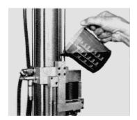
Pour oil into the duct of the type indicated on the table attached to the unit
