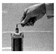
Remove filling plug situated on the top of the tank by unscrewing it anticlockwise.
